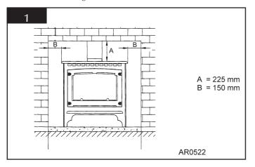
1.11 Contact a competent service engineer to carry out relevant spillage checks etc. following home improvements carried out after installation of this stove (e.g. the fitting of double glazing).
